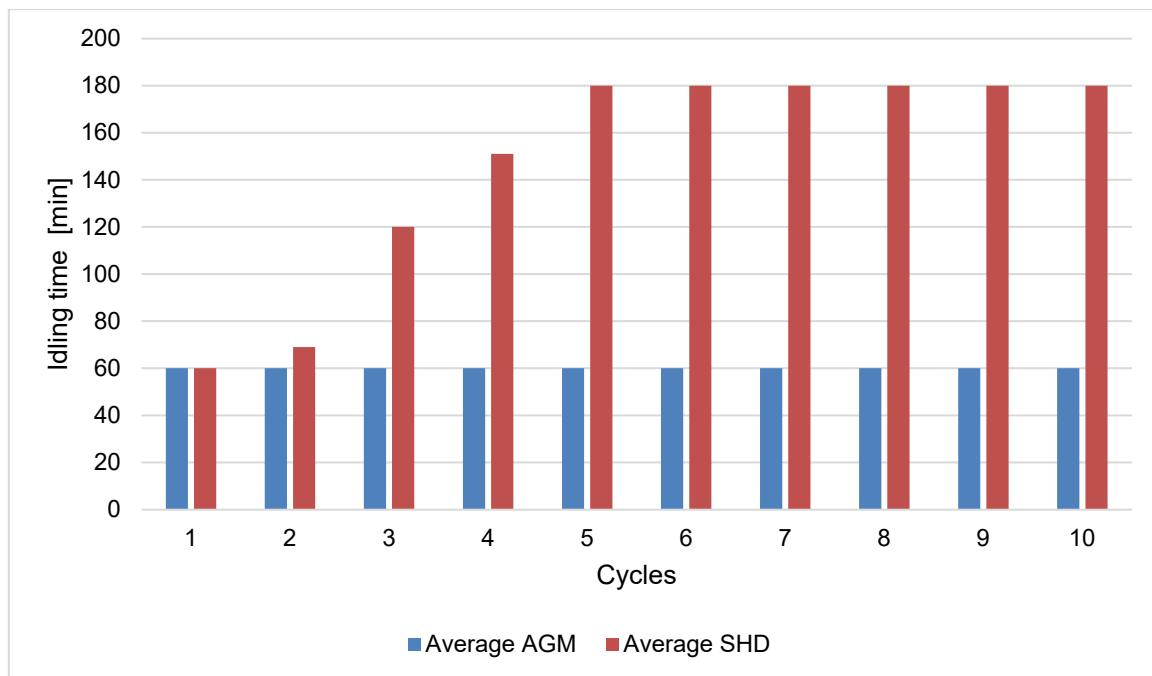
It can be concluded that average idling time of AGM batteries in weekend-rest simulation 10 cycles (after aging) is 60 minutes, while it is 148 minutes of SHD batteries.
