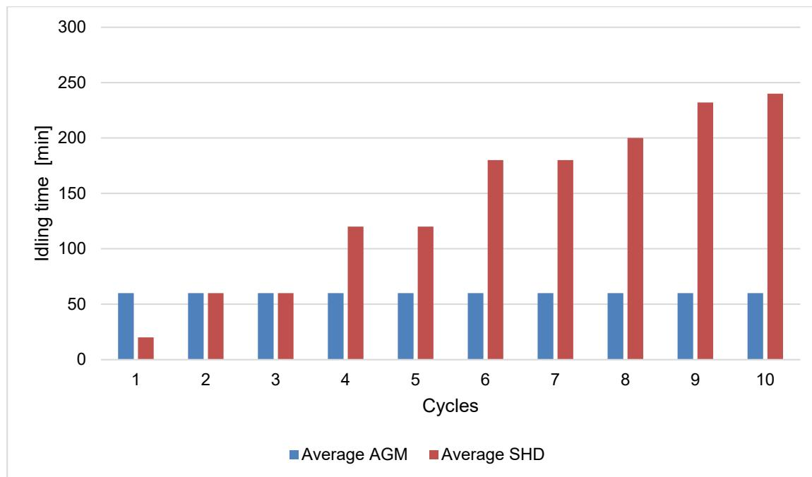
It can be concluded that average idling time of AGM batteries in weekend-rest simulation 10 cycles (before aging) is 60 minutes, while it is 141 minutes of SHD batteries.
